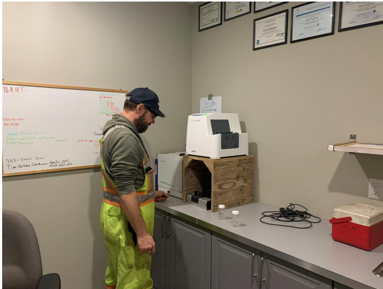
IMAGE | IN ADDITION TO WATER TESTING – IN HOUSE MICRO BIOLOGICAL ANALYSIS, WEEKLY COMPLETED BY THE WATER QUALITY TECHNICIAN.
