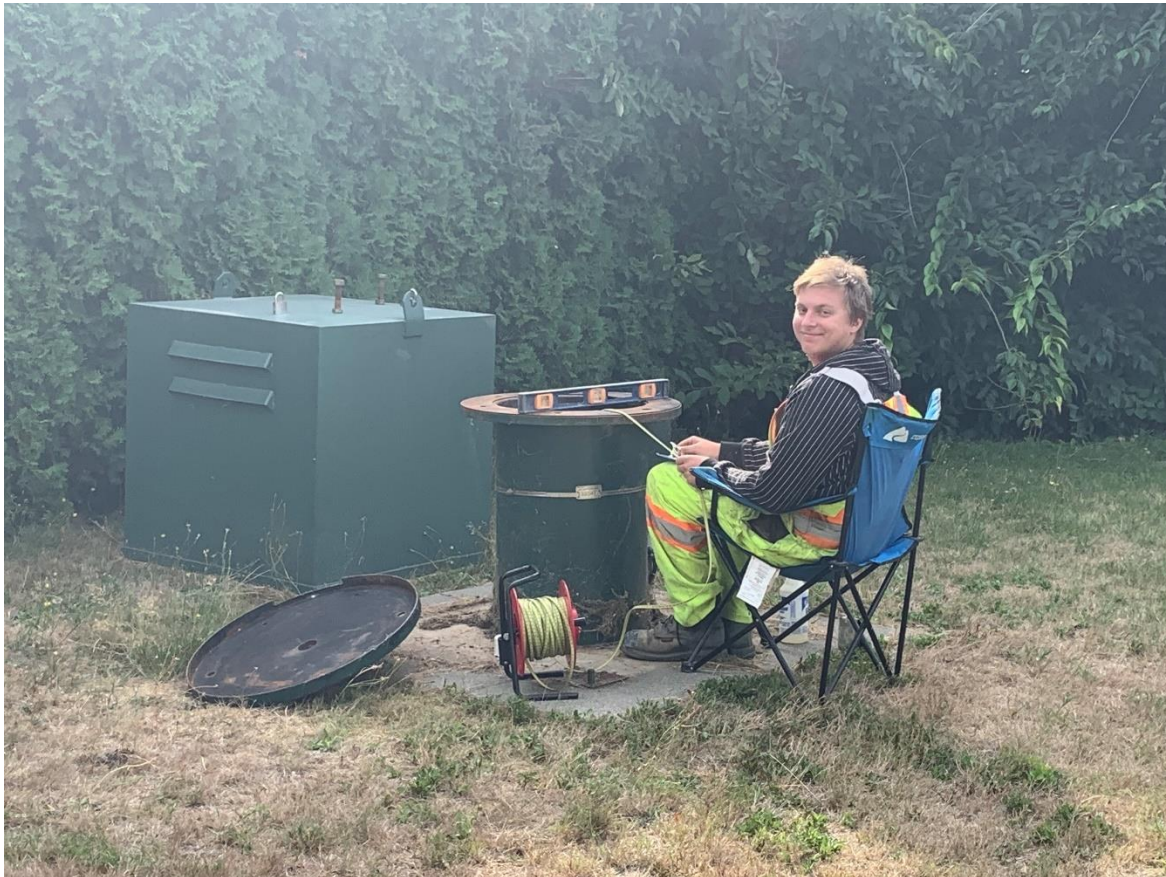
IMAGE | WATER LEVELS ARE TAKEN BY CWD STAFF DURING A STEP-DRAWDOWN PUMPING TEST.
