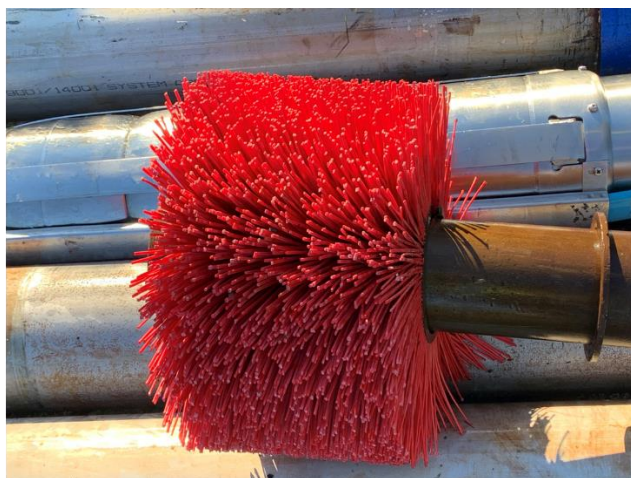
IMAGE | LEFT: THE DOWNHOLE VIDEO INSPECTION CAMERA; RIGHT: A SPECIAL WELL BRUSH USED FOR MECHANICAL AGITATION OF THE INTERIOR SURFACES OF THE WELL, PRIMARILY TARGETING THE SCREENED SECTION
